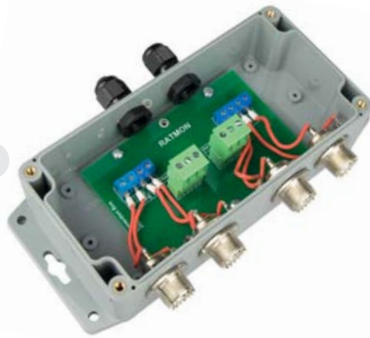
BOX-5 BNC/UHF connection box, two loops
